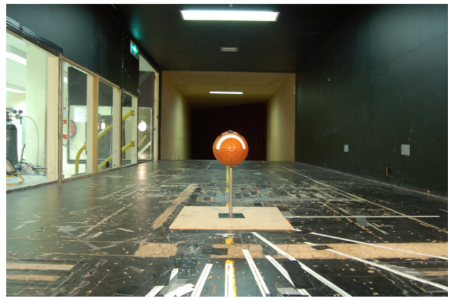
Fig. 6: Experimental setup of NCAA ball in the test section of RMIT Industrial Wind Tunnel at 0^\circ yaw
