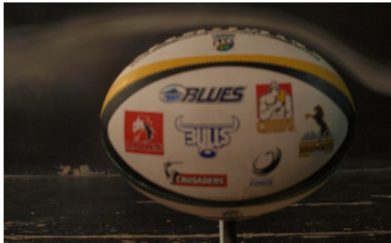
Fig. 7: Smoke visualisation at 0 degree yaw angle
