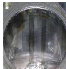
Fig 10: Mechanical damage in cylinders
