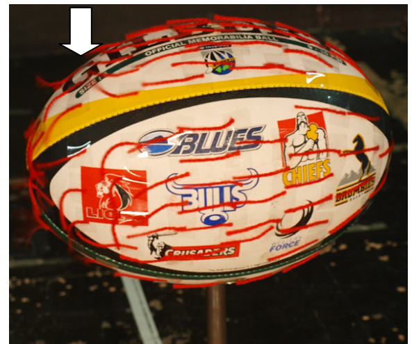
Fig. 5: Flow structure around the ball at 0^\circ yaw angle 80km/h
