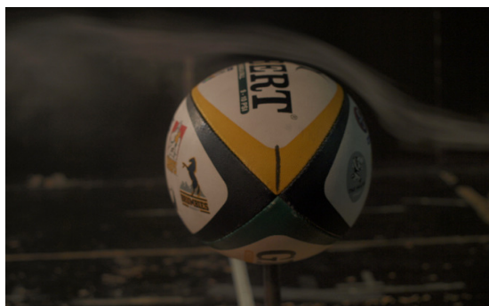
Fig. 8: Flow structure round ball at 90° and 80 km/h
