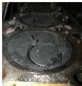
Fig 9: Carbon deposits on Nozzle and valve
