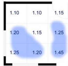
Fig. 16: Air velocity in different matrix and the comparatively comfort zone of Bed 01.
