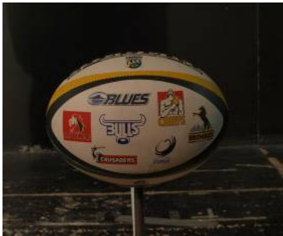
Fig. 2: Experimental set up in the RMIT Industrial Wind Tunnel with Rugby ball
