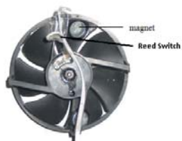
Fig 3.4.3 rotor with magnet and reed switch inside the tube
