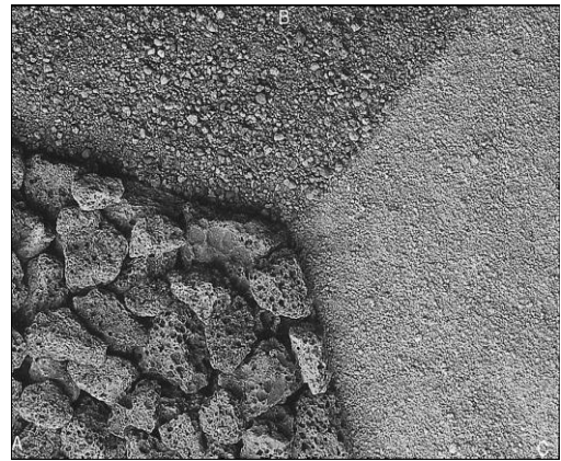
Figure 3: Slag in Various forms (Source: ACI Education Bulletin E3-01)
