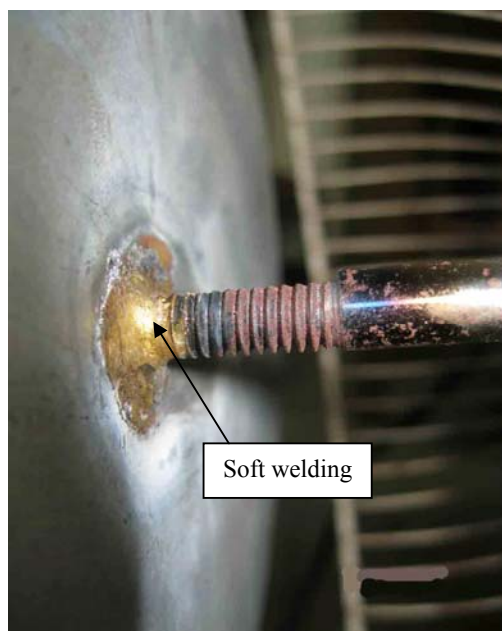
Fig.3: Soft welding of aluminium sheet with shaft
