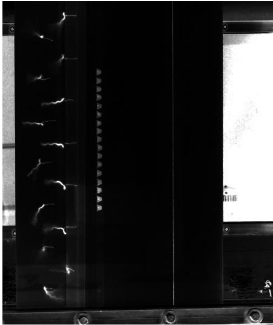
Figure: 6 triangular VG ( h=3\text{mm} , \Delta z=9\text{mm} ) 0^\circ deflected flap, \alpha = 15^\circ
